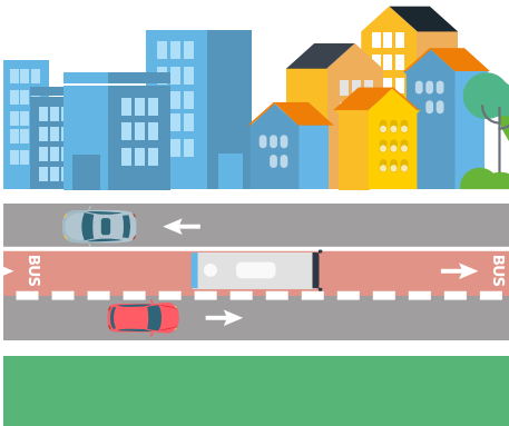
Figure 4 : Couloir bus axial unidirectionnel
